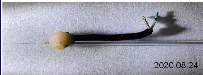
Fig. 1. Photomicrograph of a complete recording/injection electrode with connecting wire and shielding. A 30 \mu\text{m} diameter stainless steel wire was used. A. Full picture of the electrode pair. d, Dental cement; e, recording/injection microelectrode; i, injection micropipette; w, electrode wire (welded to the microwire) with shielding. Calibration bar, 5 mm. B. Enlarged view of the tip of recording/injection microelectrode in (A). i, injection micropipette; m, metal microelectrode. Calibration bar, 100 \mu\text{m} . C. Scanning electron micrograph of the tip of a representative glass-insulated microwire. t, tip of the microwire; g, insulation glass. D. Scanning electron micrograph of the tip of the microwire cut with a pair of sharp scissors. Calibration bar for (C) and (D), 10 \mu\text{m} .
